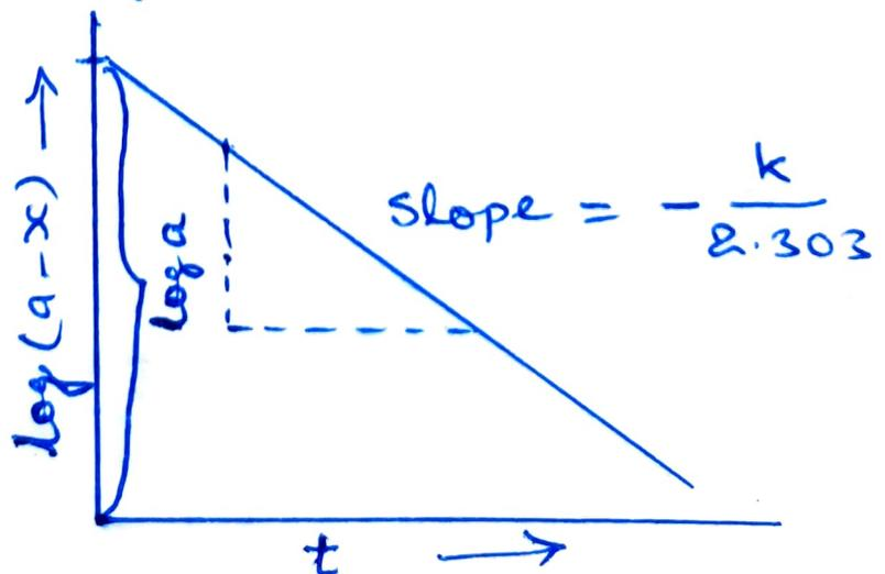
The rate constant  $k$  can thus be calculated from measuring the slope
